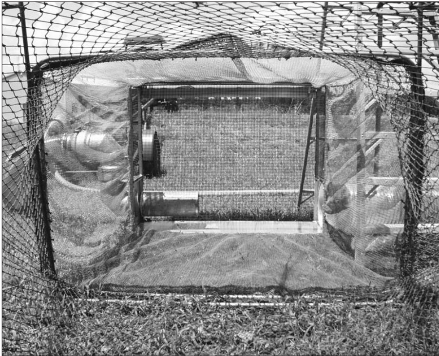
Figure 3. Inside view of the education chamber with attached live car. The 8-inch water jet (bottom left) moves the fish across the education chamber and into the 14-inch, urethane, flex-duct assembly (bottom right). The 14-inch, urethane, flex-duct assembly connects to the in-pond grader.
