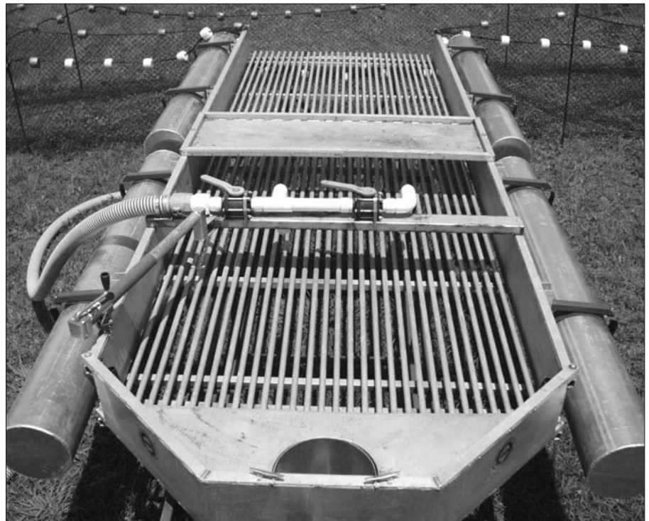
Figure 4. Top view of the in-pond grader showing the parallel bar grading surface, water jet system, and bar-spacing adjustment mechanism.
